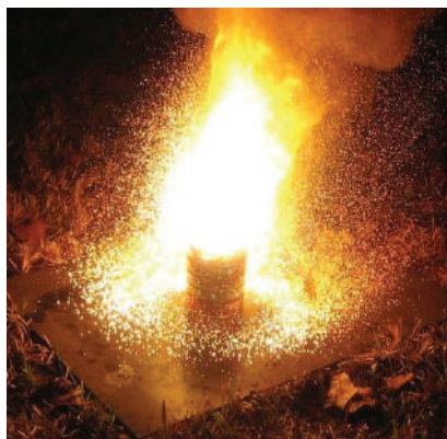
Figure 5.1: The displacement reaction between iron (III) oxide and powdered aluminium produces so much heat that iron metal is obtained in molten form.
